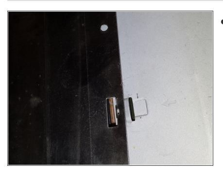
4. Carefully remove the metal clips shown below.
