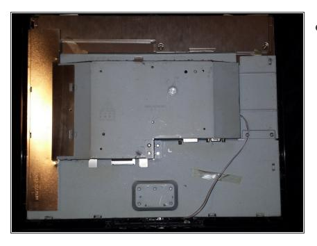
3. Now the plastic casing is able to be removed. Carefully pull apart the two pieces to reveal the metal casing as shown below. There are a few connectors you'll have to remove before revealing the power board.
