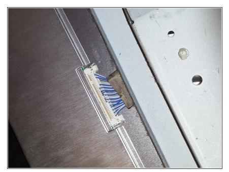
6. Remove the LCD display connector as show. You'll need to squeeze the two sides on this connector with your index finger and thumb in order to unlock it.
