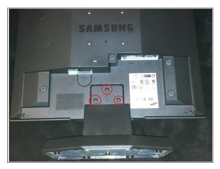
You will need a phillips screwdriver and a replacement power board which can be ordered online 1. First, place the monitor face down, then remove the plastic covering if it's on Once this is done remove the three screws shown below. Once these screws are removed, the stand is able to be removed.
