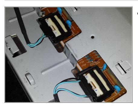
5. Once this is removed you'll need to remove the black plastic connector holders. Then remove the four connectors, I suggest you mark these to make sure they are connected back into the same location when reassembling because the monitor was known to work this way.
