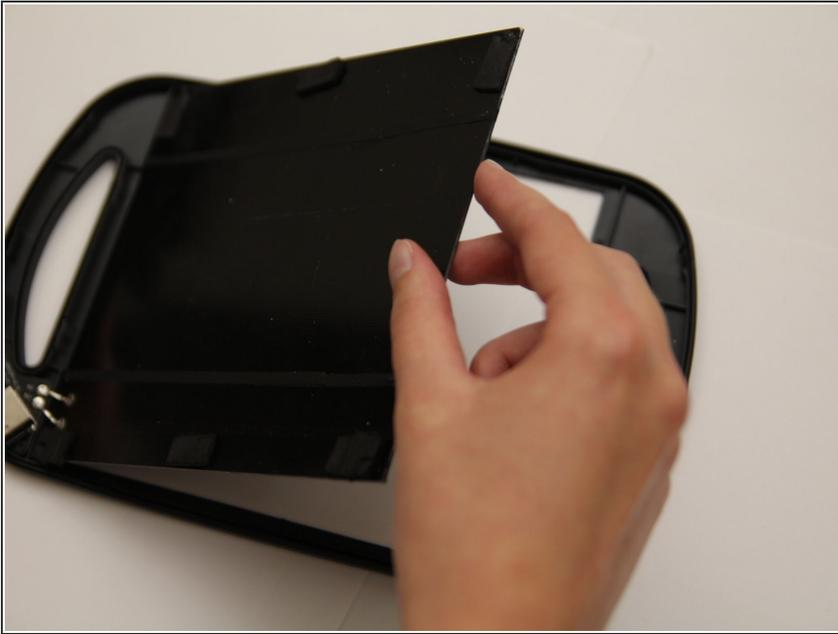
**⚠** The only thing holding the solar panel in place now is gravity, so make sure not to flip the device over! This may damage the connections.
