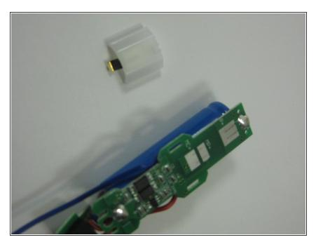
Remove the white plastic cover over the chip set allowing the battery to be taken off.
