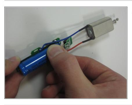
Remove the Lithium Ion Battery and replace it with the new one that you purchased.
