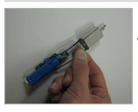
Remove the chip set, motor and battery from the plastic body. This photo shows the motor and wires connecting it to the battery.
