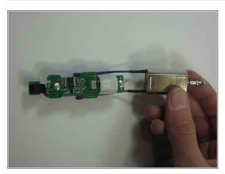
Remove the chip set, battery and motor as one piece.
