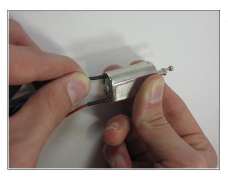
After the wires are removed and the motor is detached use the replacement motor you purchased and reconnect the wires.
