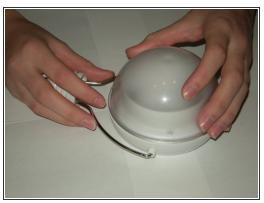
• Use one hand to hold the device still and the other to remove the lid by turning it clockwise using your index finger and thumb.
