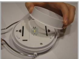
Using your index finger and thumb, squeeze the top and bottom of the plastic bezel together, and lift it off of the device.
