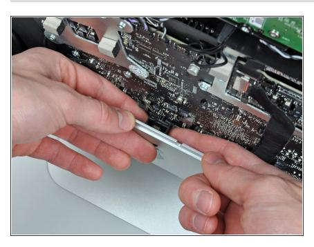
Use your fingers to lift IR sensor assembly straight up out of the outer case.
