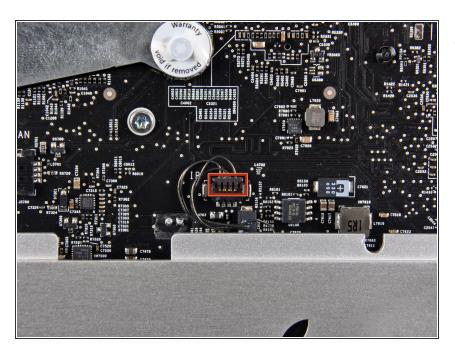
Pull the IR board connector toward the top of the iMac to disconnect it from the logic board.
