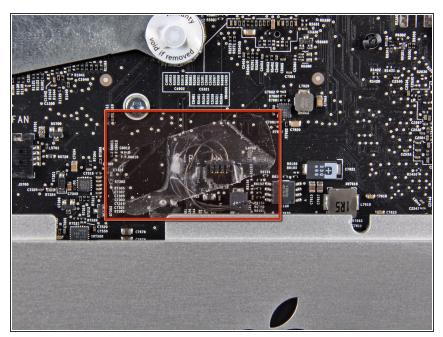
i If present, remove the piece of clear tape covering the IR board connector.
