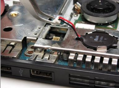
• Lift the connector from the motherboard with a pair of tweezers using a firm, upward force.
