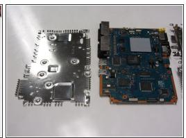
Gently separate the two metal plates from the motherboard.
