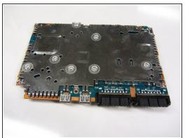
Gently lift and remove the motherboard and chassis from the outer shell.
