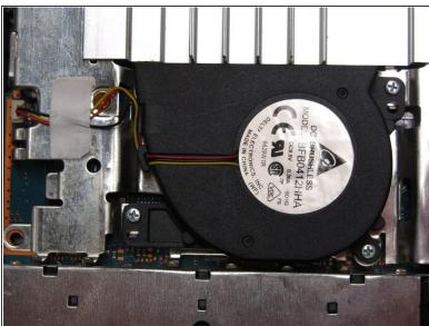
Locate the fan at the front, left section of the unit.
