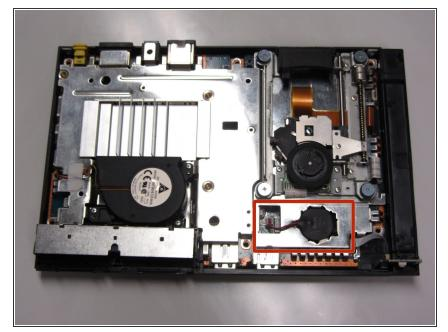
Locate the clock battery at the front, right section of the unit. The battery has a circular shape with red (+) and black (-) wires connecting to the motherboard.
