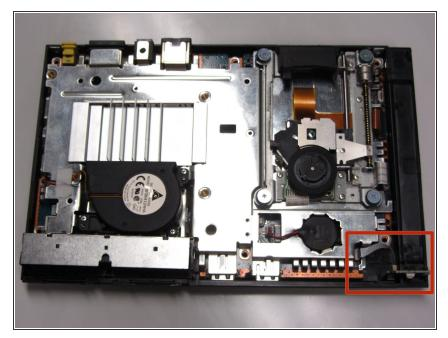
Locate the IR sensor at the front, right corner of the unit.
