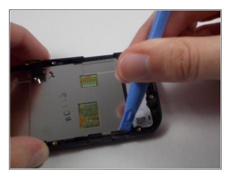
Using a plastic opening tool, detach the screen from the plastic casing of the phone.
