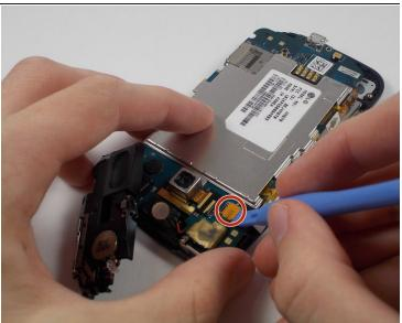
• Using your plastic opening tool, lift up the connectors on either side of the motherboard.
