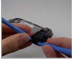
• Use a plastic opening tool to remove each area holding the parts together.
