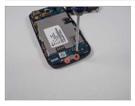
Once you have removed the antenna, unscrew the two screws located on the sides of the charging port.
