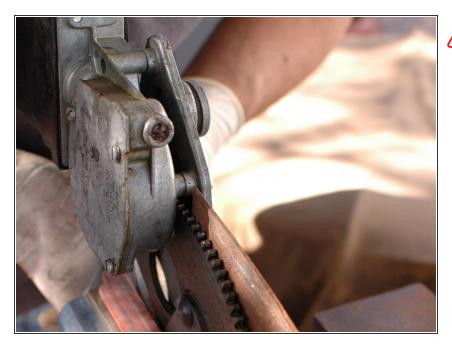
After diagnosing the regulator and finding it to be badly bent it can be secured in a vice. Be thoughtful about where you are compressing the vice on the regulator so as to not damage the various parts of the regulator.
