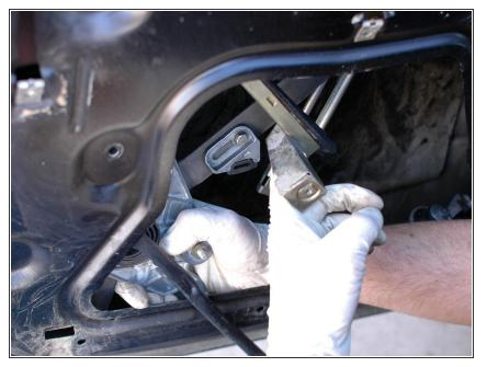
Before you can attempt to repair your rear power window regulator it must be removed from the door.
