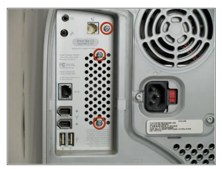
Remove these three screws that hold the motherboard fan and modem connector to the chassis.
