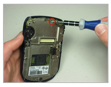
Unscrew the screw holding the back plate.
