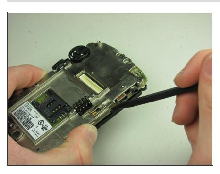
Pry off the LCD screen with spudger at the two clips.
