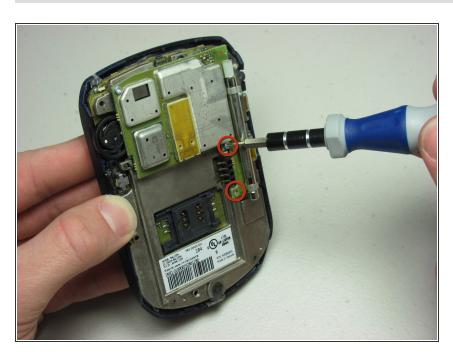
Remove the two T6 screws.
