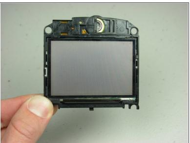
Remove the LCD screen and replace it with a new one.
