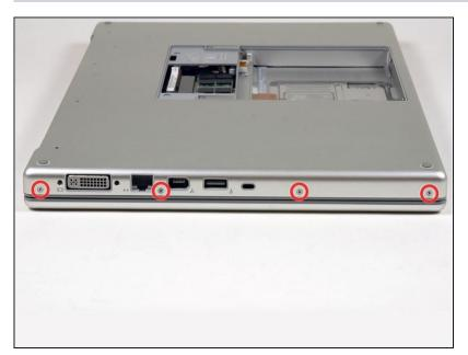
Remove the four Phillips screws on the port side of the computer.
