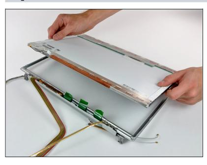
Lift the LCD out of the front bezel, minding any cables that may get caught.
