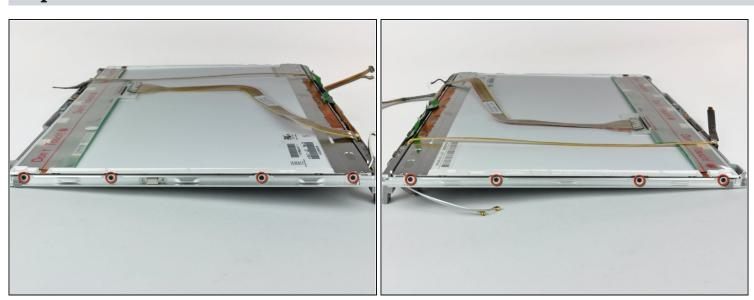
• Remove the four black Phillips screws along the left and right edges of the display (eight screws total).
