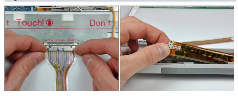
Connect the display data cable and the inverter cable connector back into their respective sockets on the original LCD assembly.
