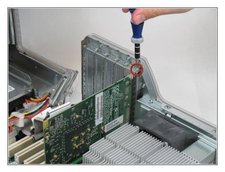
• Start by removing the screw holding the card to the chassis as shown.
