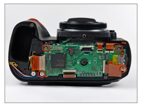
Remove the four 4.3 mm Phillips screws securing the memory compression board to the D70.
