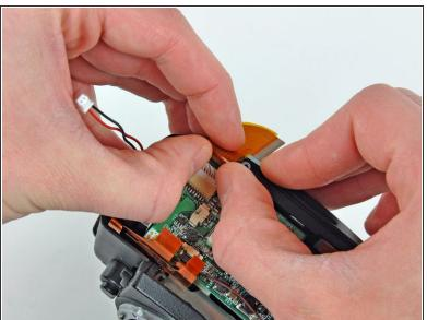
Use your thumbnails to push the CCD connector out of its socket.
