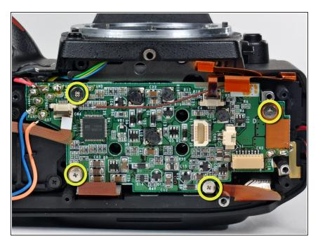
Remove the four 4.2 mm Phillips screws securing the DC/DC board to the D70.
