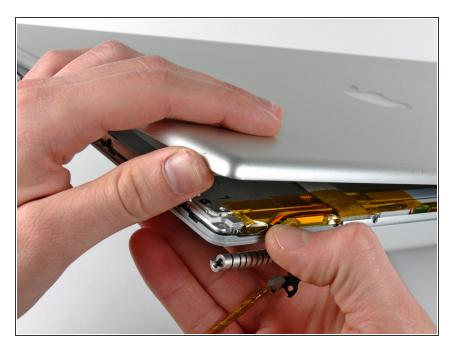
Slightly lift the recently-freed corner of the rear display bezel to separate the clips along the span of the clutch hinges.
