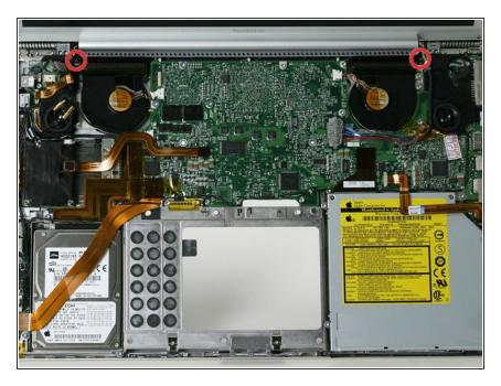
Remove one T6 Torx screw from the upper, left corner of the left fan, and one from the upper, right corner of the right fan (2 screws total).
