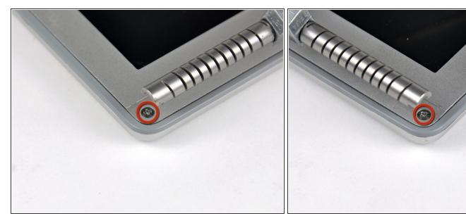
Remove the single Phillips screw from the lower left and right corners of the display.
