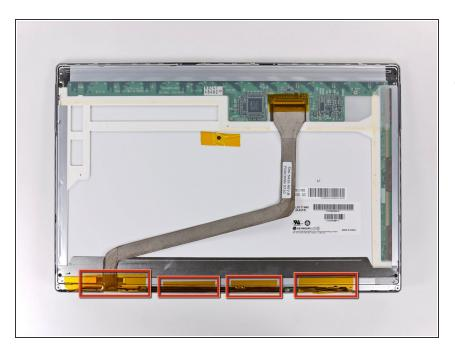
Remove the pieces of tape along the lower edge of the display that are covering the opening of the clutch hinges.
