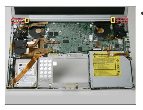
when reassembling the display, check to see that the hinges are seated properly before reinstalling the 8 screws of the two hinges. There is a metal phalange on the inside end of each hinge assembly that must be pointed downward and fit into a slot below the inside edge of the hinge. If not, the inside end of each hinge will sit too high and the plastic retaining bracket for the wiring will not sit down properly.
