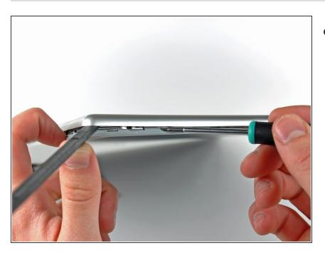
Repeat the previous procedure to release the clips along the left side of the rear display bezel.
