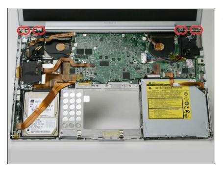
From each complete hinge assembly, remove two Torx T6 screws from the outside of each set, leaving two remaining in the middle of each hinge. On each side, the two screws closer to the edge of the computer are shorter than the two screws closer to the center of the computer. Then remove the two inner screws from each hinge assembly. There are 8 screws total.
