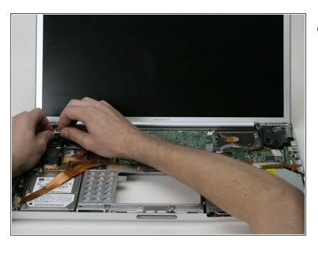
Disconnect the Airport antenna cable at the gold connector, making sure you pull only on the gold metal portion of the connector.
