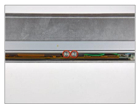
Remove the two 10.3 mm T8 Torx screws securing the center of the clutch hinges to the front bezel.
