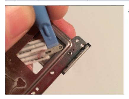
Further take apart the slide mechanism by removing the spring with a plastic spudger.
