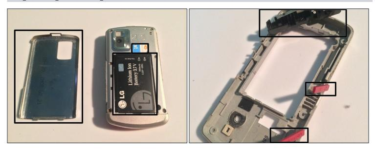
• It is possible to remove and swap out these parts before reassembly: battery cover release button, grounding clip, charging and SD card slot covers, plastic/metal framework
