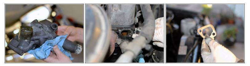
• **Required**: In order to remove your short cooling bypass hose you will first need to remove the thermostat housing. The thermostat housing gasket will need to be replaced, with fresh gasket sealant, at the end of this job. For guidance on removing the housing and replacing the gasket [invalid guide link]
