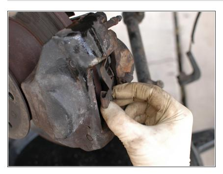
Place the retaining spring back on top of the pads.
