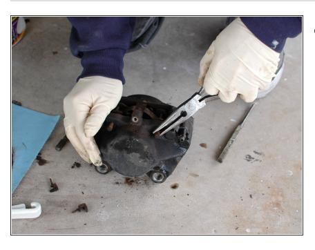
Once you have punched the pins out part of the way they may be pulled the rest of the way out with a needle nose plier.
