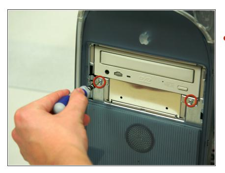
Remove the two screws on the front of the drive with the Phillips #1 screwdriver.
