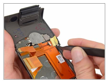
Peel back the yellow tape covering the cable connector on the back of the casing you removed.
