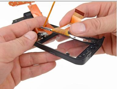
• Lift and remove the LCD from the rear case.
