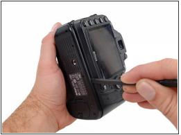
Using a spudger, separate the bottom panel from the rear case just enough to clear the two clips on the rear casing in the next step.
