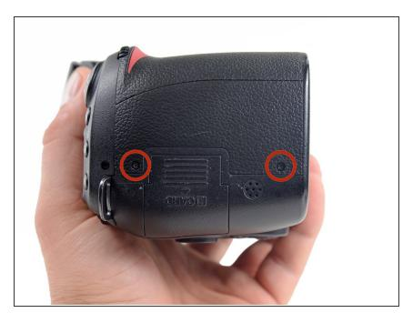
Remove the two 6.4mm Phillips screws on the right side of the camera, near the SD card slot.
