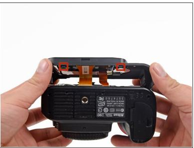
Lift the rear case off of the back of the camera.
