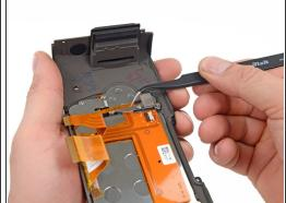
• Using the spudger, rock the connector back and forth to disconnect the cable.
