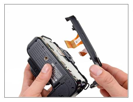
Separate the rear casing from the camera.
