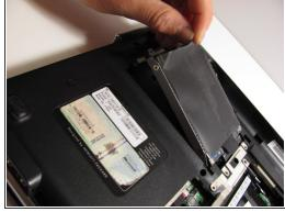
Use the Mylar tab to lift the hard drive up, and then slide it to the left to release it from the hard drive bay.
