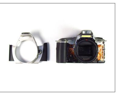
Remove the front panel by pulling away from the side with the lever.
