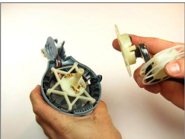
Remove the two parts of the retracting wheel.
