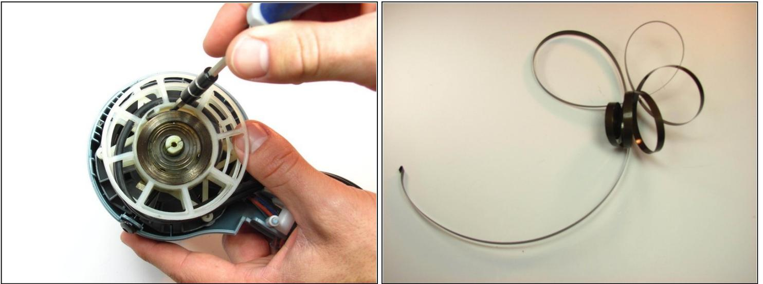
★ **When removing the coil, make sure it stays wound up. It could very easily pop out, and you would have to wind it all the way back up and try to squeeze it back into the slot when you reassemble the dryer.**
