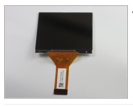
You should now be able to remove the LCD screen. Replace it with a new screen.
