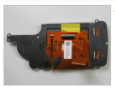
Detach the ribbon cables on the LCD casing.
