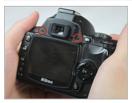
Remove the two visible 6.0 mm
