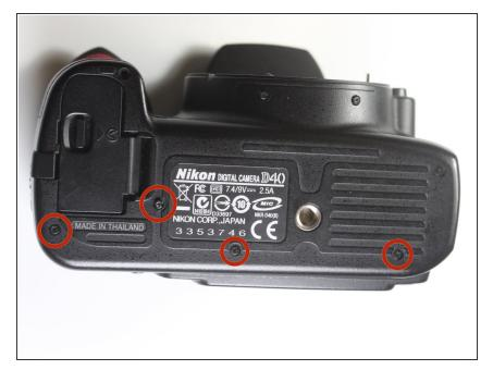
Remove the four highlighted 3.0 mm
