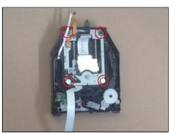
• Carefully remove the plastic shell, paying attention to the cable that runs through it for the 4-cables model.
