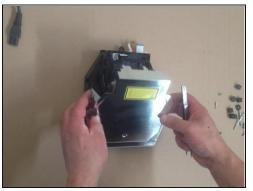
Disassemble the upper metal shield by first unscrewing the 3 Phillips screws.
