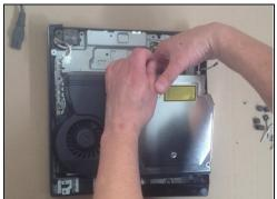
• Separate cables, unscrew the screw and remove the Blu Ray drive.
