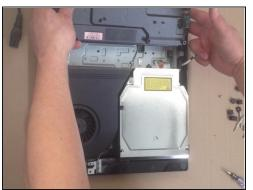
• To remove the power supply, first disconnect the two cables, then the 2 Phillips screws. Then lift it upwards.
