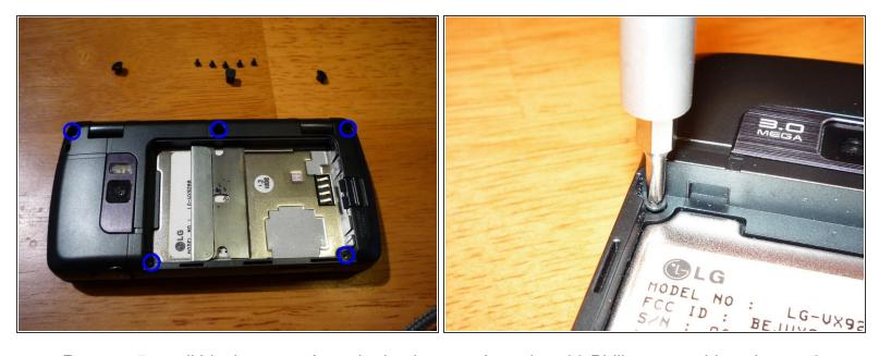
Remove 5 small black screws from the back cover. I used a #00 Philips screwdriver, but a #0 should also work as well.
