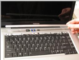
Remove the plastic strip above the "F" keys using the spudger by placing the small end of the spudger under the strip and lifting up.
