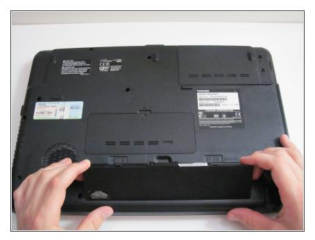
Remove the battery by placing your finger in the middle groove and lifting up.
