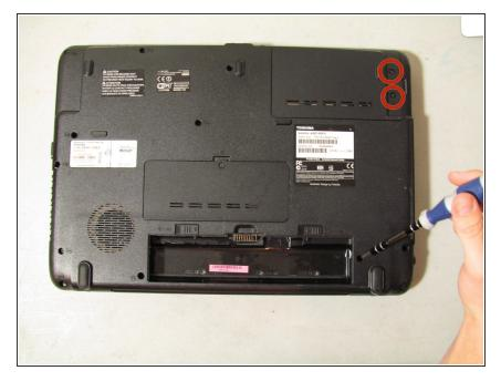
Remove the two Phillips #1 6mm screws from the backside of your computer using a Phillips #1 screwdriver.
