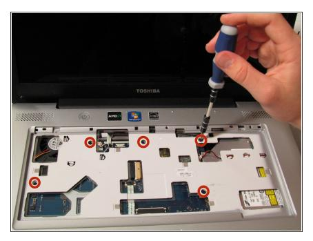
Remove the five Phillips #1 10mm screws underneath the keyboard using a Phillips #1 screwdriver.
