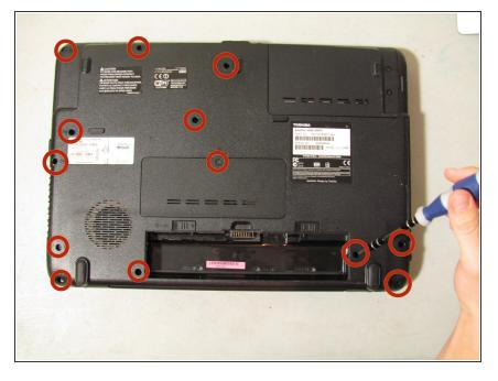
Remove the 13 Phillips #1 10mm screws from the backside of your computer using a Phillips #1 screwdriver.
