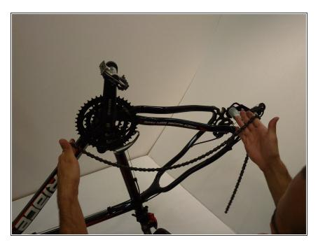
Once the chain is separated, remove it from the bike by pulling one end.
