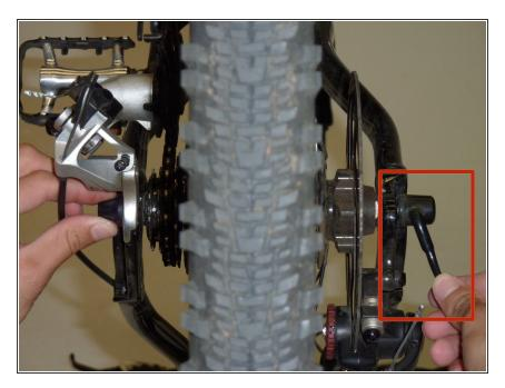
Begin loosening the tire by turning the quick release handle.
