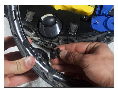
Pull gently on the bottom of the sensor to remove.
