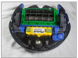
With a Phillips #1 screwdriver, remove the ten 12mm screws located along the bottom of the bumper.
