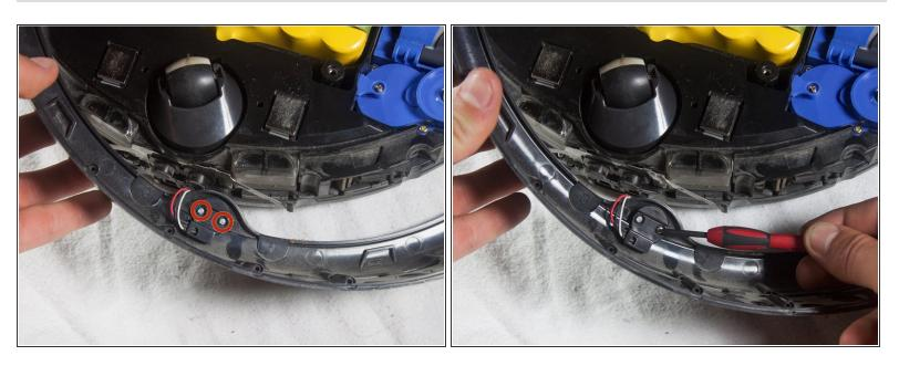
Remove the two 5mm screws located near the center of the bumper using a Phillips #1 screwdriver.
