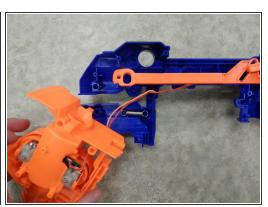
Remove the two 9.0 mm Phillips screws.
