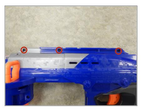
Remove the three 9.0 mm Phillips screws holding the top latch of the Nerf Gun together.
