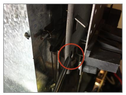
Use a flat-head screwdriver to separate the metal flap from the metal plate.
