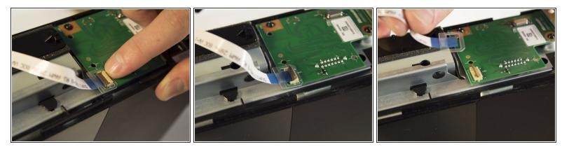
• Find the brown section where the ribbon cable enters the green board. Flip the brown part up and pull out the plastic tab at the end of the ribbon.
