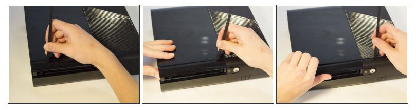
• Beginning on the left side without the grate, run the spudger along the crevice until you've reached the grated part, while holding the part that's being separated as you go.
