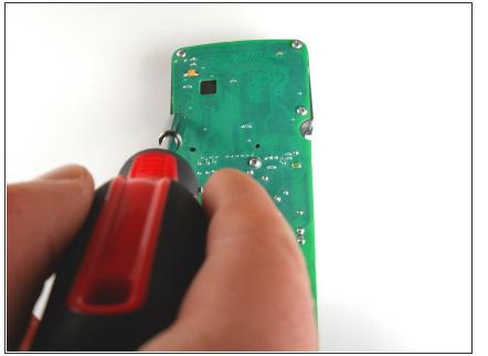
Use the Phillips #1 Screwdriver to remove the five silver 11 mm Phillips #1 screws attaching the green circuit board to the grey plastic internal cover.
