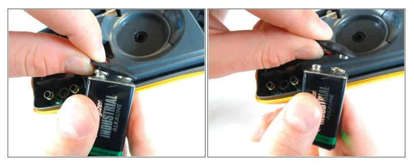
$\bigwedge$  Only pull on the metal snaps and battery. Pulling the cords may damage them.
