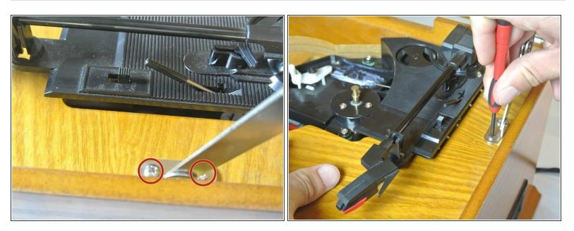
• Remove the two 12 mm screws that attach the hinge to the box.
