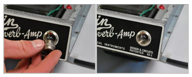
• Remove the cap covering the light bulb by unscrewing the cap counter clockwise.
