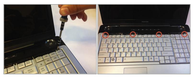
Use a #1 Phillips screwdriver to take out the four 4mm Phillips #1 screws that were underneath the plastic strip.
