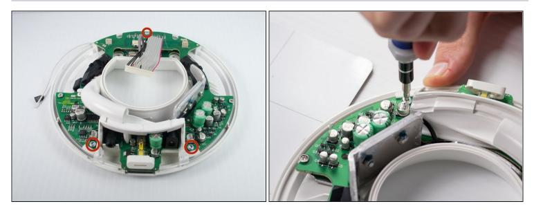
• Remove the three 1 cm T-10 Torx screws.
