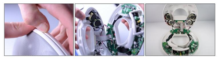
• Open the device along its seam.
