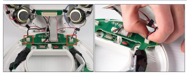
• Locate and disconnect the two molex connectors found on either side of the ribbon cable connector on the bottom half of the device.
