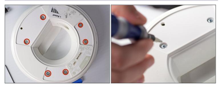
• Remove the six 1cm T-10 torx screws on the bottom of the device (found under the rubber pads) using a T-10 Torx screwdriver.
