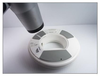
Use a heat gun (set to low) to apply heat to one of the rubber pads until you can easily remove the pad. This step takes around 5-7 minutes.
