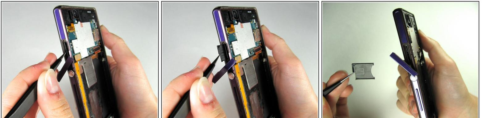
⚠ To avoid damage to the SIM card, be careful when removing and handling it.
