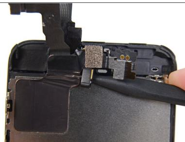
Slide the point of a spudger under the microphone to lift it out of its recess in the display assembly.
