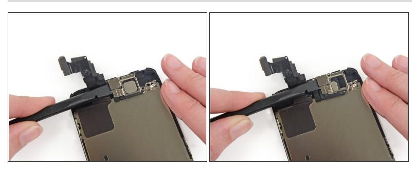
• Use the flat edge of a spudger to push the earpiece speaker bracket off the display assembly.
