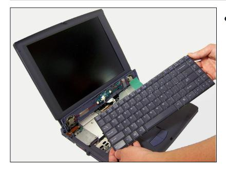
• Your keyboard is now safety detached. Necessary repairs or replacements can be made from here.
