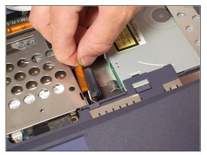
Carefully detach the harness from the CD/DVD drive. Use your fingers if possible, but if not carefully use a pair of tweezers to detach the harness. Take care in not bending any of the pin connections.
