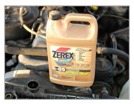
If your coolant is low, top it off with a mix of about 50/50 distilled water to coolant. Only use a proper coolant for these cars, either the Genuine Mercedes coolant or one that is specified and formulated for the application.
