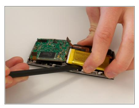
Use the spudger to carefully pry up the battery. The battery is attached with a few spots of glue, so it may not move at first.
