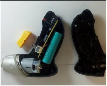
• Using a plastic opening tool, separate the case in two to expose the internals of the cordless screwdriver.
