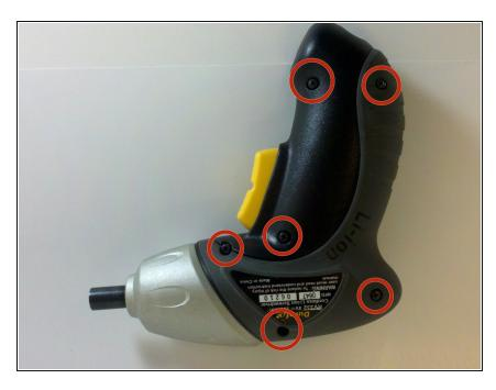
Remove the six 13 mm case screws with a #0 Phillips screwdriver from the side of the power screwdriver.
