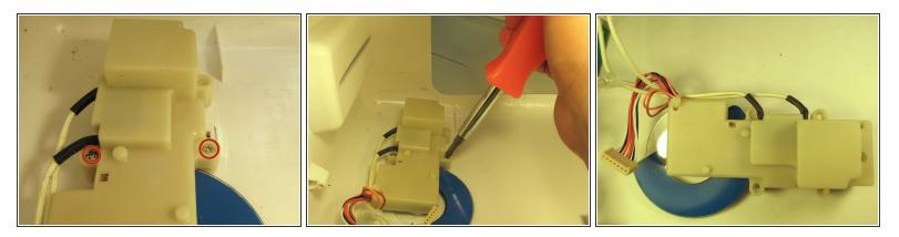
• Remove the screws to detach controls from the plastic shell of the toaster.
