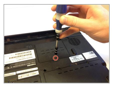
Using a Phillips-head screwdriver, unscrew and remove the screw holding the RAM slot cover in place.
