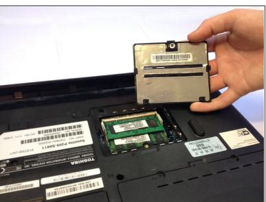
Lift and remove the RAM slot cover.
