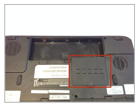
Locate the RAM slot cover on the bottom of the laptop. The RAM slot cover is located near the battery slot.
