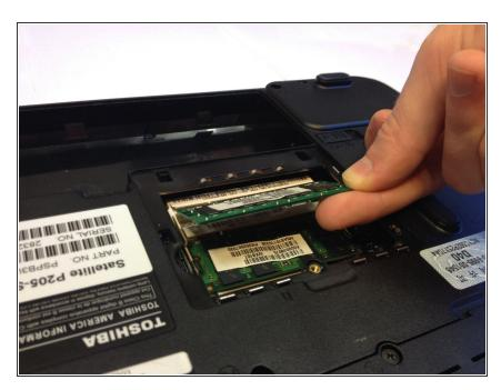
Using your fingers, remove the RAM chip by gently pulling it out of the RAM slot.
