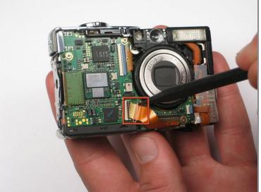
Pull the retaining clip up with the spudger or your finger and remove the ribbon from the socket.
