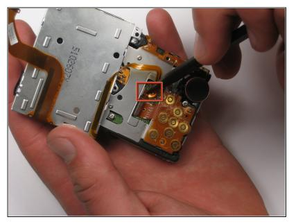
Pull the back light ribbon from it's socket to remove the LCD completely. There is a little hole you can stick the spudger into to help release the ribbon.
