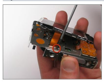
Remove the last screw holding the tripod mount to the case. The LCD ribbon threads under the mount, so upon reinstallation, the ribbon will need to be threaded through before the mount is reattached. Take note of the tripod mount orientation.
