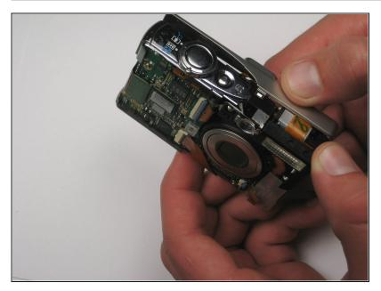
Take hold of the inside of the camera, and gently pull away from the back casing.
