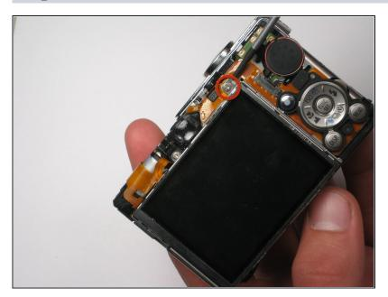
Remove the screw at the top right of the screen.
