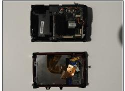
Using the spudger and tweezers if needed, remove the ribbons from the computer chips.
