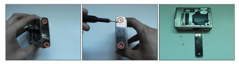
• Using the Phillips #00 screwdriver, unscrew the two screws on the side of the camera.
