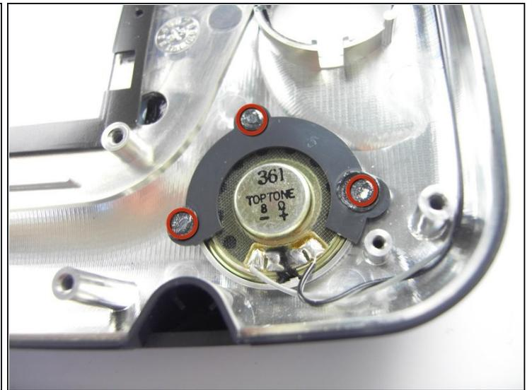
⚠ Removing the plastic holding the speaker to the case may permanently detach the speaker.
