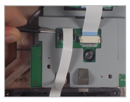
Unlock the second cable shown in the photo by using the pointed tweezers to move the lock upward on both sides of the cable.
